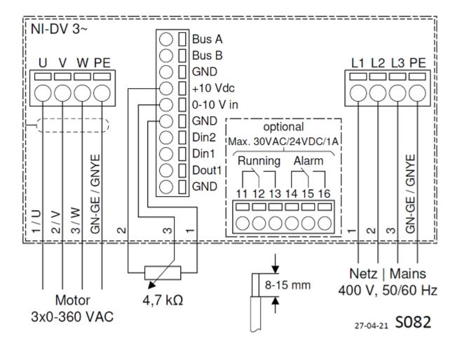
Wiring diagram for connection to: mains - VSD - motor
